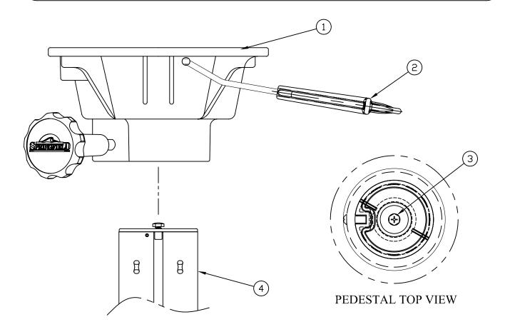
After placing your Springfield Marine Slide or Swivel (Item #1) onto the pedestal (Item #4) verify that the pedestal adjustment handle (Item #2) is functioning properly.
